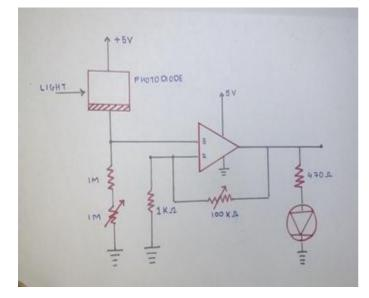
The switching point is determined by the pin 6 (inverting input terminal). The light intensity on the photodiode controls the switching process of the reference voltage. The 2K pot is connected to pin 7 (non-inverting terminal); It is used to set the input threshold voltage of any desired value by comparing the input voltage of pin 6.
